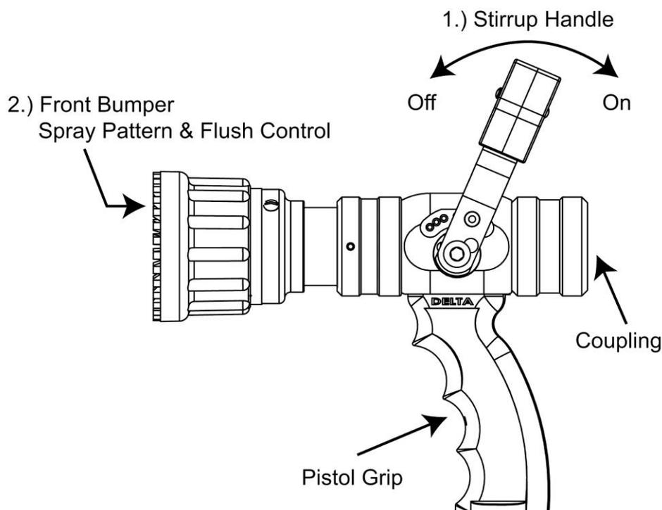
The H500 ST Nozzle has full water stream pattern control, from straight stream to wide spray/fog settings, fully adjustable by simple rotation of the front bumper. An additional 'flush' setting is available by counter-clockwise rotation of the bumper to enable the operator to clear debris that may have entered the nozzle inlet via the water stream.
